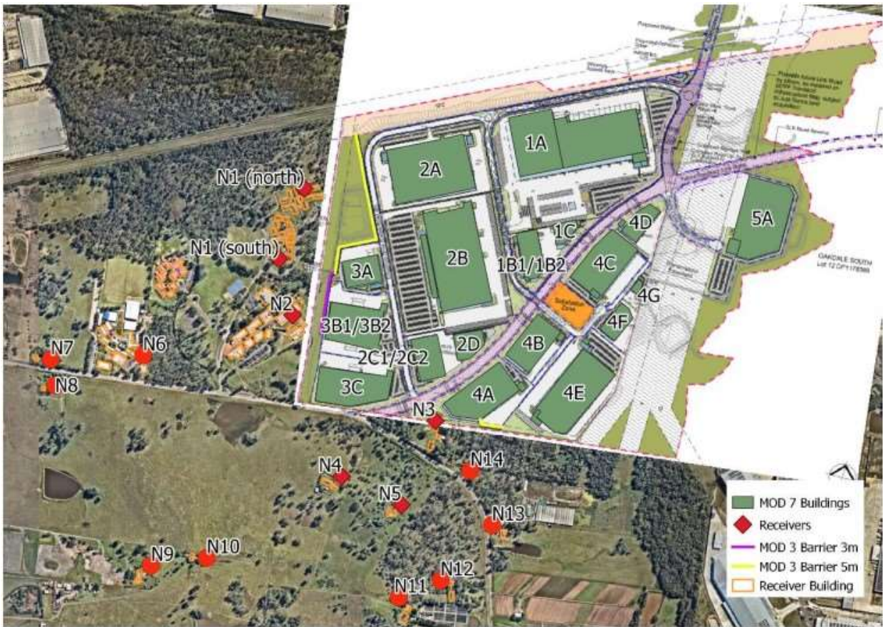
Figure 6: Noise Receivers and Noise Wall Locations
