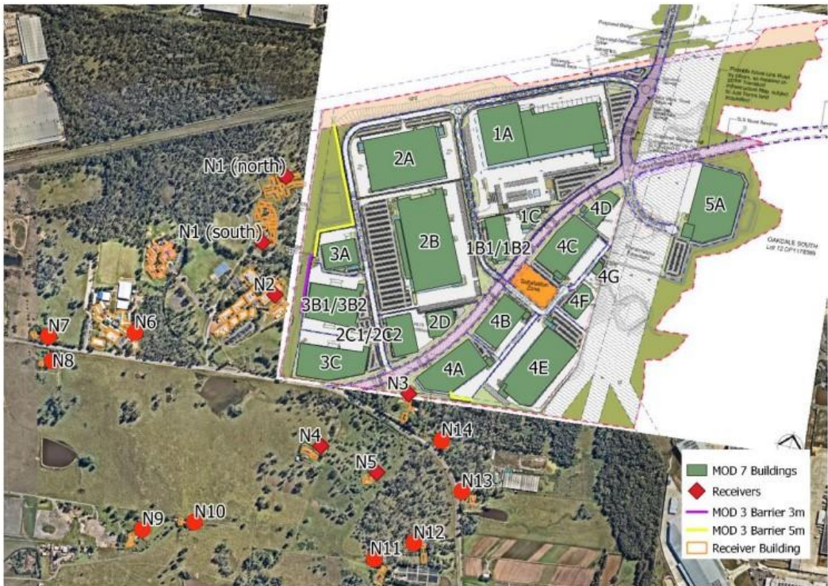
Figure 6: Sensitive Noise Receivers and Noise Wall Locations
