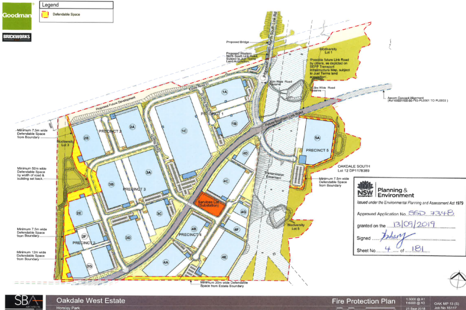
Figure 2 - Oakdale West Estate 2019 Approved Masterplan showing Defendable Space widths to the future buildings.
