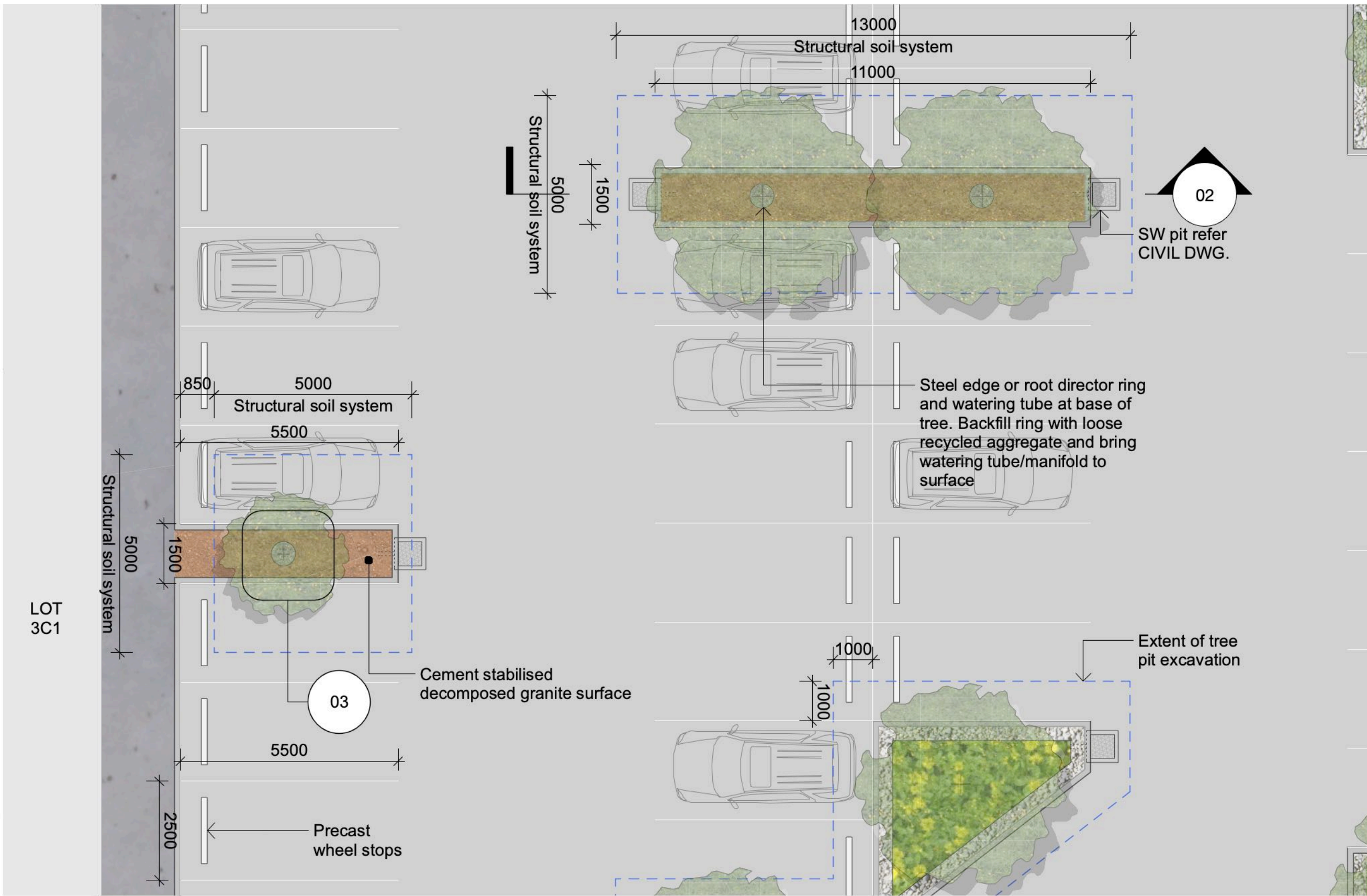
01 Carpark Tree Pit System Detailed Plan - Scale 1:100 @ A1
