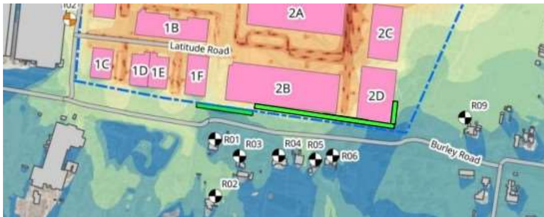
Figure 8: Temporary noise barrier approximate location – Stage 2 Development
