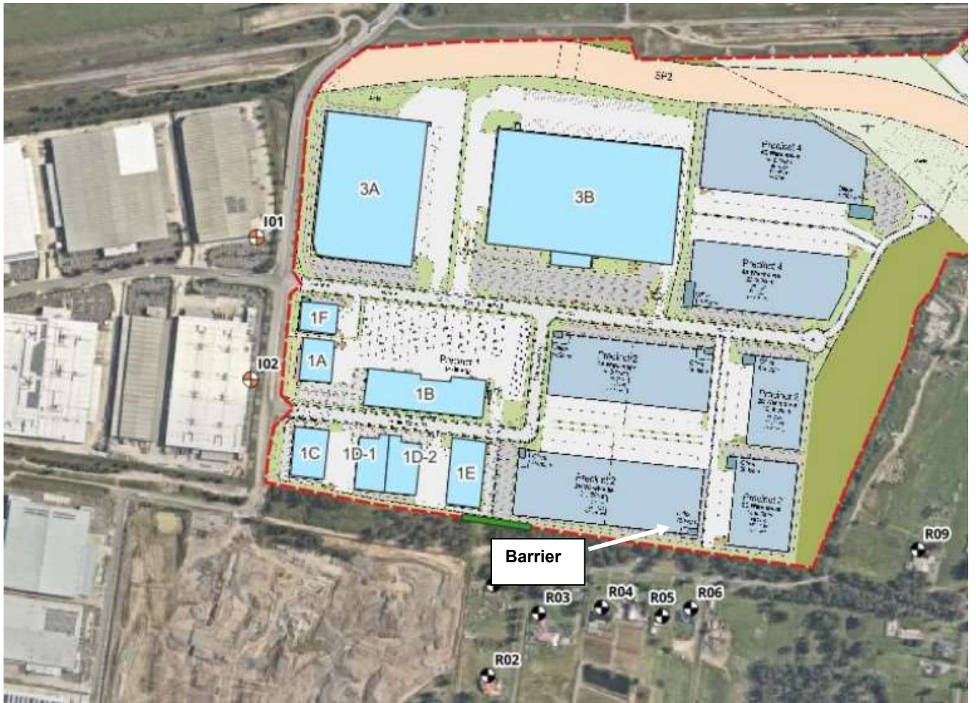
Figure 8: Temporary Noise Barrier Location – Stage 2 Development
