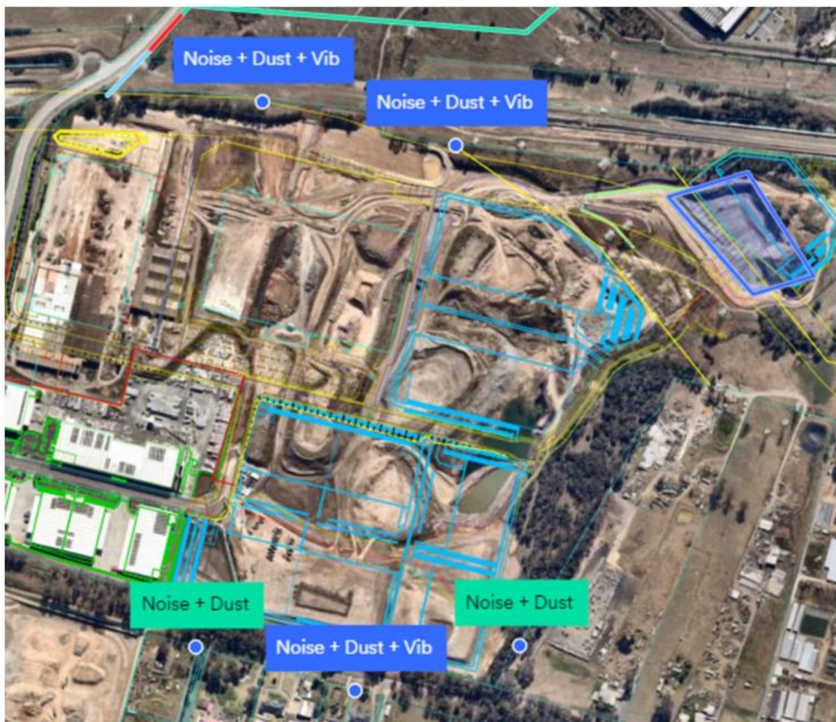
Figure 8 Indicative SiteHive Real-Time Monitoring Locations
