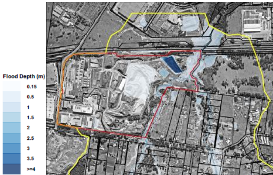
Figure 4.8 – Extract of Drawing A3 (Page 10 of the ‘Oakdale East Flood Assessment’ prepared by BMT) which depicts the ‘Peak Flood Depth - Developed Scenario - 1% AEP Flood’
