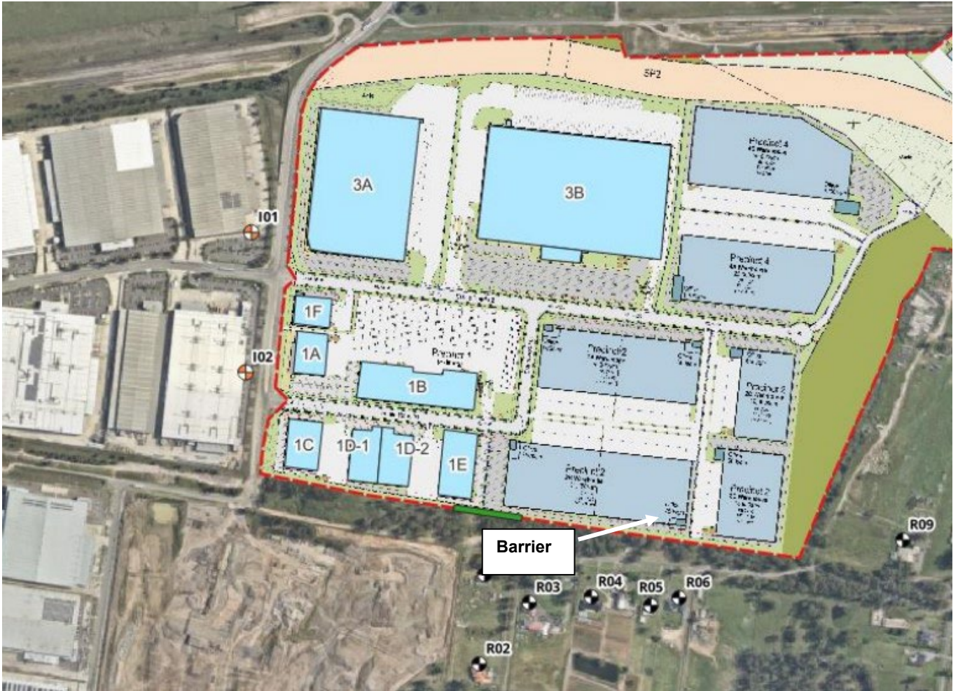
Figure 8: Temporary Noise Barrier Location – Stage 2 Development
