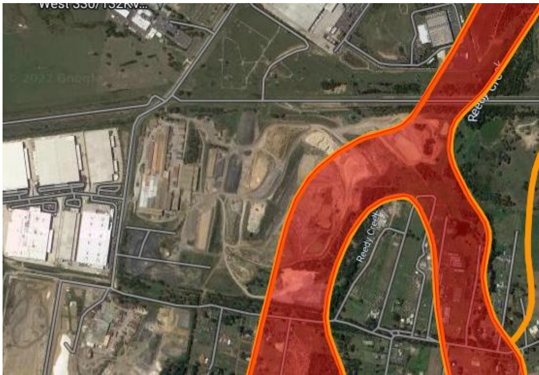
Figure 4.1.2 – Extract map of the occurrence of the 'South Creek' soil landscape unit from NSW Office of Environment & Heritage website resource 'eSPADE'
