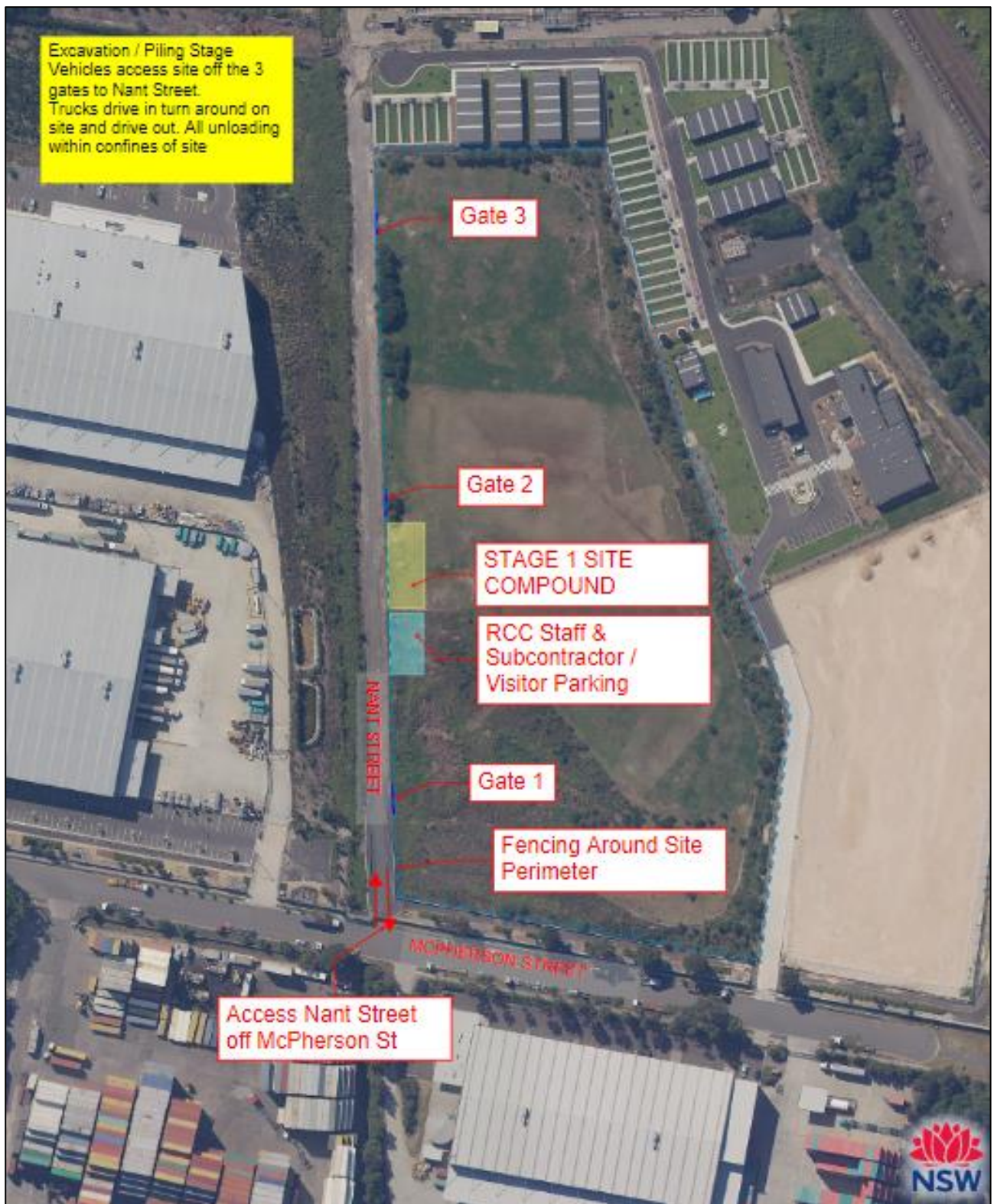
Figure 5: Proposed Site Access Gates and Construction Site Layout
