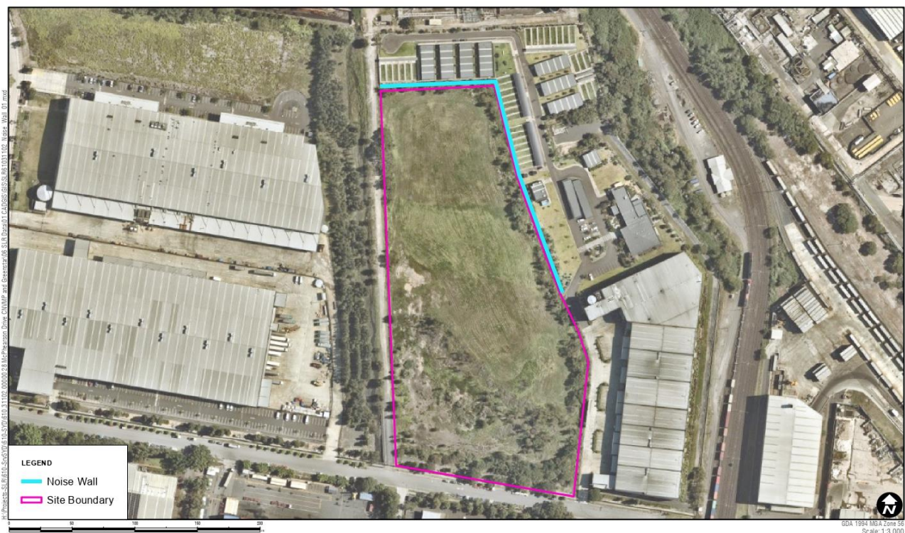
Figure 5 Noise Barrier Position
