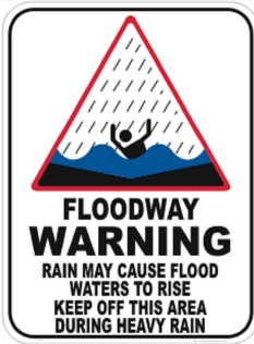
FLOODWAY WARNING SIGN NTS SUGGESTED SIZE 600mm x 450mm TO BE PROVIDED NEAR FLOOD WATER DEPTH BOARDS IN SUITABLE AREA T.B.C ON SITE
