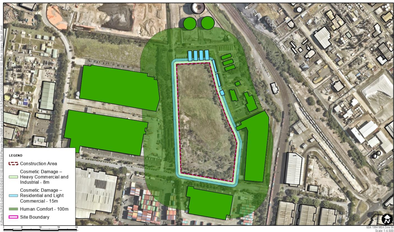
Figure 4 Construction Vibration – Vibratory Roller (12 t) and Impact Piling Rig
