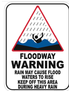
FLOODWAY WARNING SIGN NTS SUGGESTED SIZE 600mm x 450mm TO BE PROVIDED NEAR FLOOD WATER DEPTH BOARDS IN SUITABLE AREA T.B.C ON SITE
